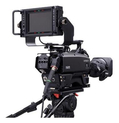
Supporting multiple HD formats (upto 1080/50p), the Z-HD6500 camera's design offers content producers and broadcasters visual quality that reaches new heights through a combination of three 2/3-inch UHD-resolution CMOS image sensors with global shutter to
