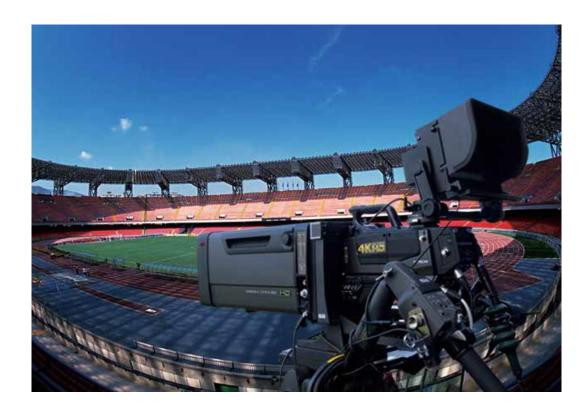
Hitachi's SK-UHD4000 system 4K color camera can be used with existing 2/3-inch format ENG and Studio/Field lenses without the use of an optical-mechanical adaptor between camera and lens.
